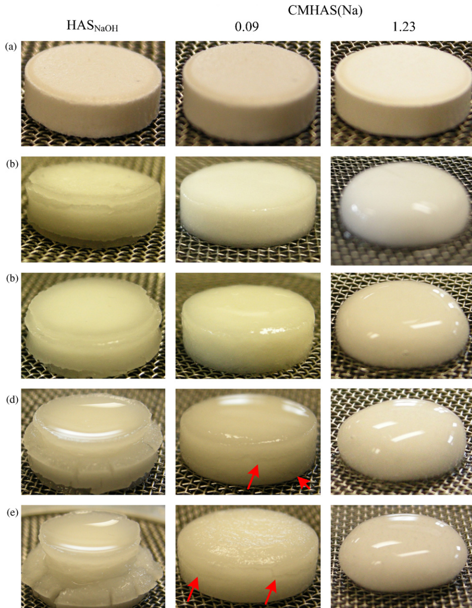
Fig. 7. Physical appearance of typical tablets of HAS NaOH and CMHAS(Na) with a DS of 0.09 and 1.23 incubated in SGF after: (a) initial (0 h), (b) 3 h, (c) 5 h, (d) 7 h and (e) 9 h.
